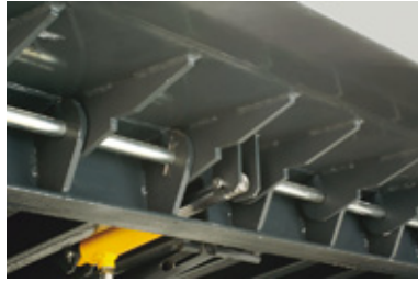
Self-cleaning reinforced hinges.
